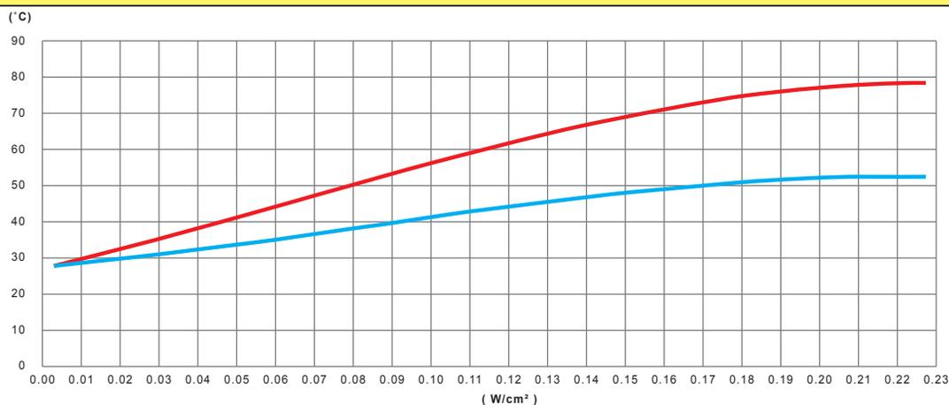
Variation, in function of the power in W/cm<sup>2</sup> of the silicone heating tape, of the temperature of the wall of a **tubo in PVC vuoto, non isolato termicamente.**
